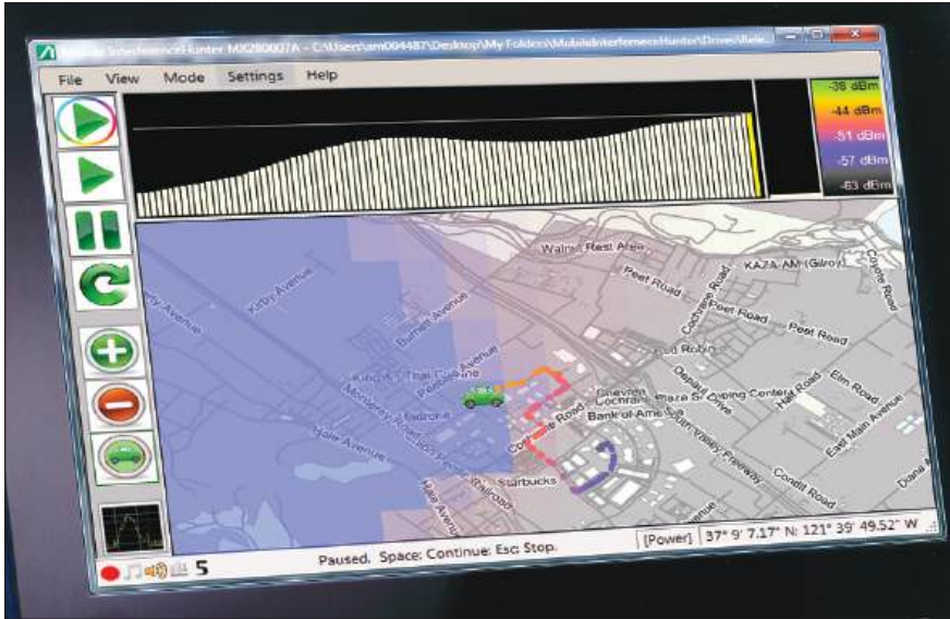
Figure 1. Mobile InterferenceHunter MX280007A on Windows® PC Tablet with Spectrum Master™ Device in Vehicle
