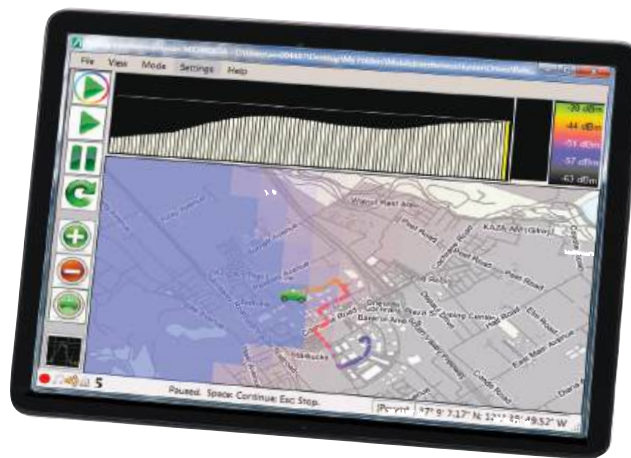
OpenStreetMap™ Displayed on Windows PC tablet. InterferenceHunter Screen Capture. Dots Shown Along Drive Path are Colored according to Signal Strength.
