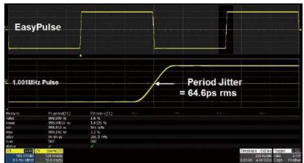
When a Square/Pulse waveform is generated by DDS, there will be a one-clock-jitter if the sampling rate is not an integer-related multiple of the output frequency. SDG2000X EasyPulse technology successfully overcomes this weakness in DDS designs and helps to produce low jitter Square/Pulse waveforms.
