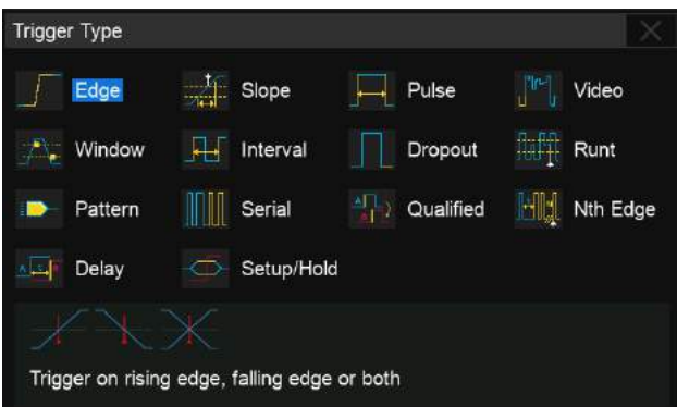
Edge, Slope, Pulse width, Video, Window, Runt, Interval, Dropout, Pattern, Qualified, Nth edge, Delay, Setup/Hold time, and Serial trigger.
