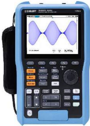
Front panel of the SHS800X series
